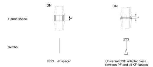
An additional sealing gasket and bolt of a size corresponding to the length of the spacer should be planned in for flange couplings for the most regularly used PDG type glass spacers. The additional length in mm is marked by entering option "L" after the item number. Examples of this are also shown in the following table. More detailed information on the above-mentioned flange couplings and sealing gaskets can be found in chap. 2 "couplings".
