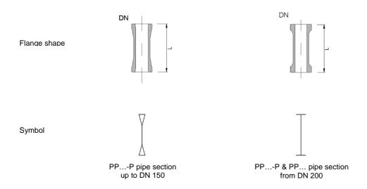
You can find more information on types of pipe end which are dependent on nominal diameter in chap. 10 "technical information" as well as on the corresponding flange couplings and sealing gaskets in chap 2 "couplings".
