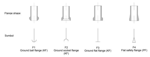
To help identify the ends of flanges the type of flange is entered at the end of each item number, for example "F44" for pipe sections in the PF system. The order of the flange details is also important in clearly identifying many structural components. The numbering DN 1, DN 2, etc is used for these structural components on the relevant catalogue drawing. Flange types should be entered in the item number according to this order, for example "F121" for the T piece in the example below.
