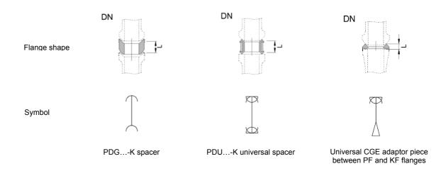
An additional sealing gasket and bolts of a size corresponding to the length of the spacer should be planned in for flange couplings for PDG type glass spacers, which are most frequently used. The additional length in mm is marked by entering option "L" after the item number. Examples of this are shown in the following table. More detailed information on the above-mentioned flange couplings and sealing gaskets can be found in chap. 2 "couplings".
