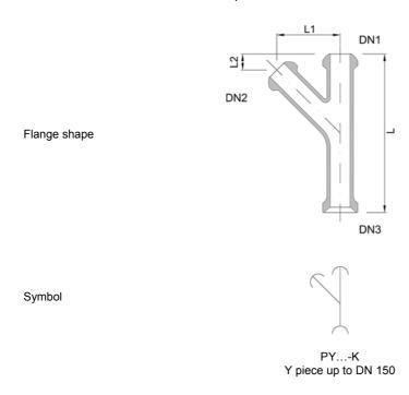
We will be happy to deliver optional extras such as coatings and further flange combinations for the KF system. For this you need to add the optional extra digits to the item number as given at the end of the chapter. To request specific flange combinations enter the flanges you require in order, DN1, DN2, ..., according to the outline above.
