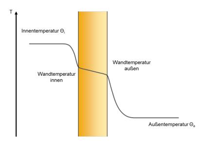
figure 10.2: temperature shape across a glass wall for Borosilicate Glass 3.3
