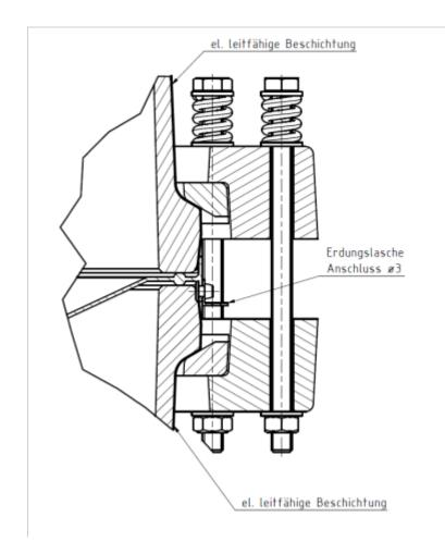
figure 10.3: Exemplary connection with a conductive coating, conductive gasket and earthing connection
