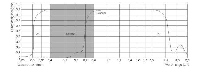
figure 10.1: Transmission curves for Borosilicate Glass 3.3
